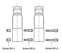
Screw 3E1-1 & screw 3E1-2: for the first station Screw 3E1-3: for the second and other station
